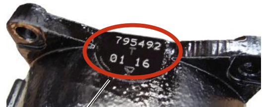
Drivebox Assembly Part No. Example: 795492 and Date Code Example: 01 16
