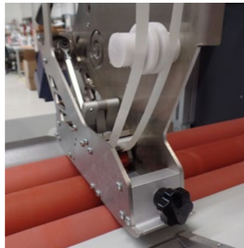
Ability to apply two rolls of tape on the same applicator for close parallel tape strips
