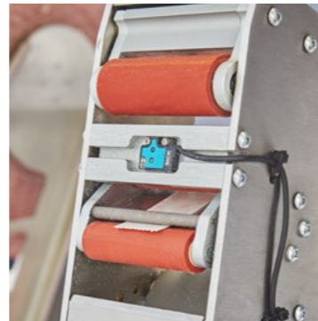
The photocell “sees” many types of substrate material: black, transparent, reflective.. and allows easy placing of tape around die-cut holes
