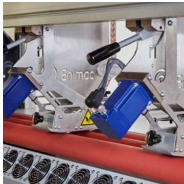
“Automatic zero” on the applicator motors speeds up the set-up process
