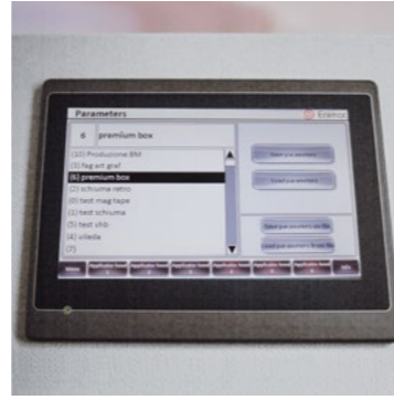
Multi-job software capable of saving machine settings for up to 100 jobs
