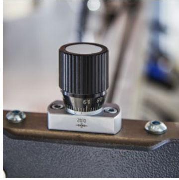
Precise micrometric adjustment of the applicator beam height accommodating substrates up to 15mm thick
