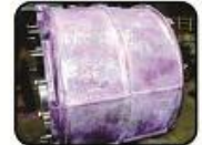
SOLID CAST STAINLESS STEEL BODY / CASING / WITH DPT TEST
