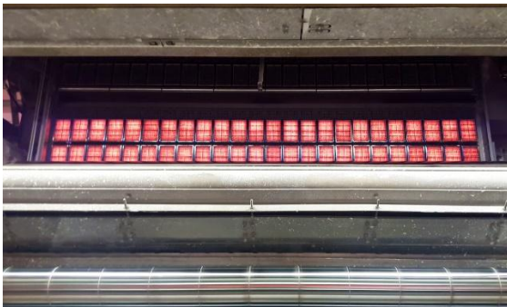
GemDryer® made of 4 rows of 24 Gem9E emitters
