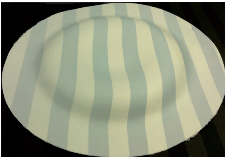
Fig. 2: Hydroforming test body with projected fringe pattern (Source: TU Darmstadt – PMV)
