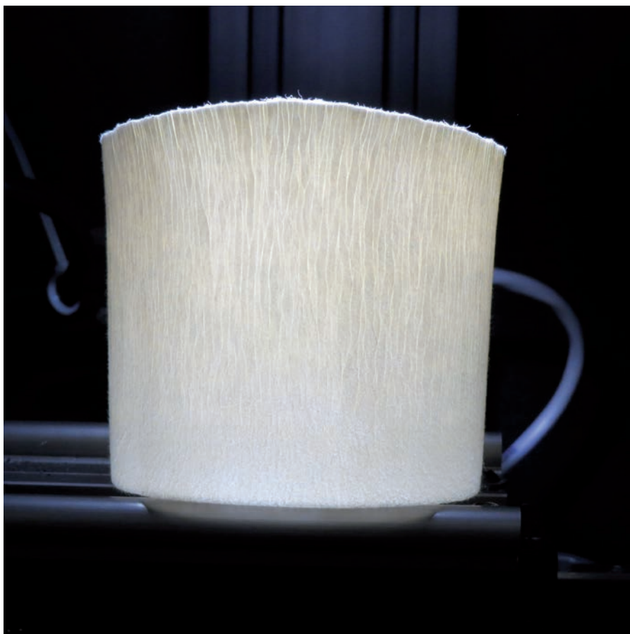
Fig. 3: Cylindrical body made from paper by deep drawing (Source: TU Dresden – VAT)
