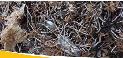
The Belgian paper manufacturer VPK Packaging Group produces several tonnes of waste material every day in the form of pulper ropes, which in the past were collected by a local waste management company. In future, the pulper ropes generated will be internally processed and separated. To achieve this, the packaging specialist has turned to the XR3000C – a machine that has already proved itself many times as a single-pass solution for processing pulper ropes.
