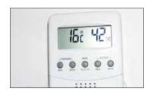
It was therefore planned for the temperature of the room to be maintained between 16-18°C and the RH at 45%  $\pm$  5%. The Bry-Air Dehumidifiers had a nominal capacity of 100 CFM. The temperature and humidity are consistently monitored (three readings are taken in the duration 12 hours, and minimum maximum for each 24 hours) and reported. A generator backup ensures that power to the vault is never off for more than 5 mins.
