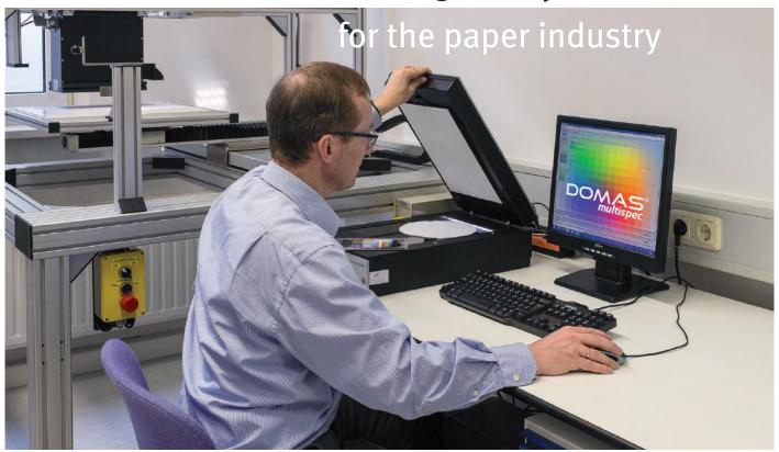
DOMAS *multispec* is a modern modular imagae analysis system, that can record, process and analyse multispectral data, recorded using a scanner or camera, to supplement optical images. At the moment available are formation measurement and NIR chemical imaging; more modules are to be underway.
