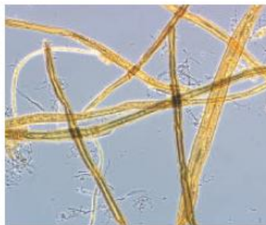
Very fine crill particles attached or detached from the fibers are resolved with ultraviolet light in the CrillEye measurement
